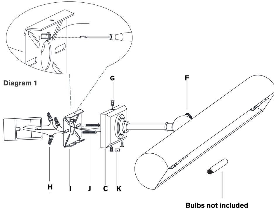
10. Install fixture body (**C**) to hardwire mounting plate (**I**) and secure with screws (**G**).
