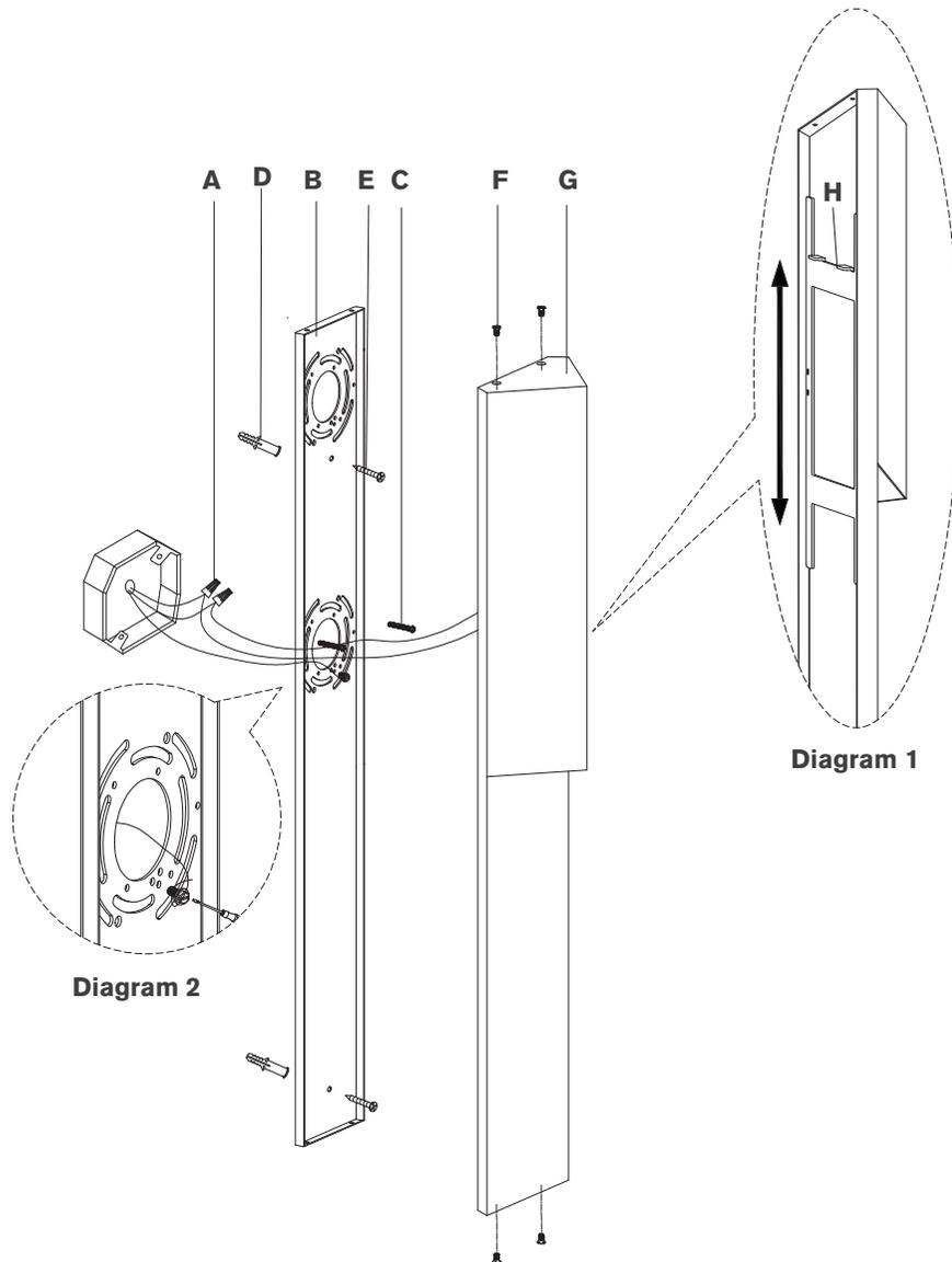
10. Make sure all wire connections are tight, then carefully tuck into the junction box.
