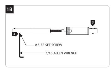
**3** Loosen (Do Not Remove) all five #6-32 set screws with the 1/16 Allen wrench to clear the holes.
