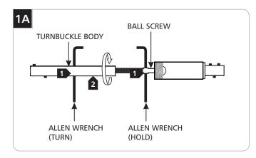
Insert one Allen wrench into inline turnbuckle body hole and another one into the ball screw hole.
