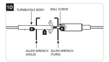
6 Insert one Allen wrench into inline turnbuckle body hole and another one into the ball screw hole.
