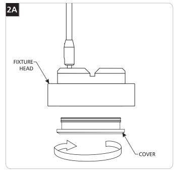
**NOTE:** While installing or replacing lens and/or optics, it is recommended to do so with the fixture head facing downward to hold items in place within the cover during installation.
